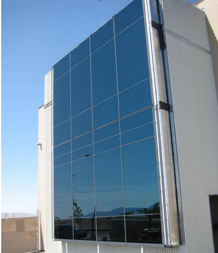
EN-WALL System Mockup Installed in EN-WALL's in-house test chamber in Las Vegas, NV, USA
